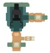
•**Dual check valve (DCV):** This device consists of two independent check valves that are connected in parallel. It prevents backflow by allowing water to flow in only one direction.
