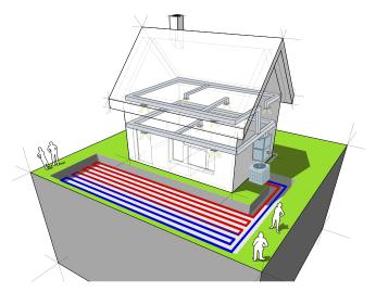
**Ground-source heat pumps** use underground pipes, known as ground loops, to extract heat from the earth. These loops are filled with a heat-transfer fluid that absorbs heat from the ground and carries it to the heat pump. Ground-source heat pumps offer high efficiency and consistent performance since the ground temperature remains relatively stable throughout the year. However, they require more upfront investment because ground loops must be installed.
